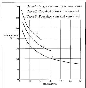
Figure 1. Nominal Efficiency of 'Model Quality' Worm Gearing
