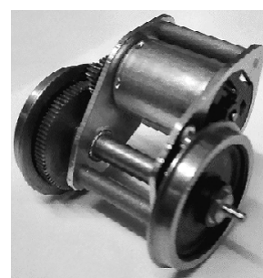
Photo 7.1 Axle and motor assembly
