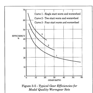
mounted worm gears should fall within a band 5% above or below the average efficiency curve illustrated. If a particular gearing combination efficiency falls below that band it needs to be inspected to discover where the fault lies. It is very important to ensure that slight backlash is present in a worm drive and that the gearbox frame does not distort under load. In extreme cases distortion of the box can cause total lock-up of the drive.
