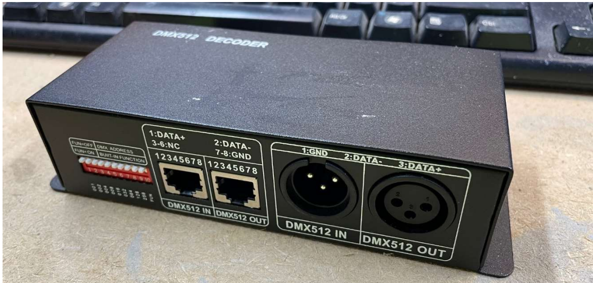
High current 12V LED DMX decoder showing the XLR interfaces
