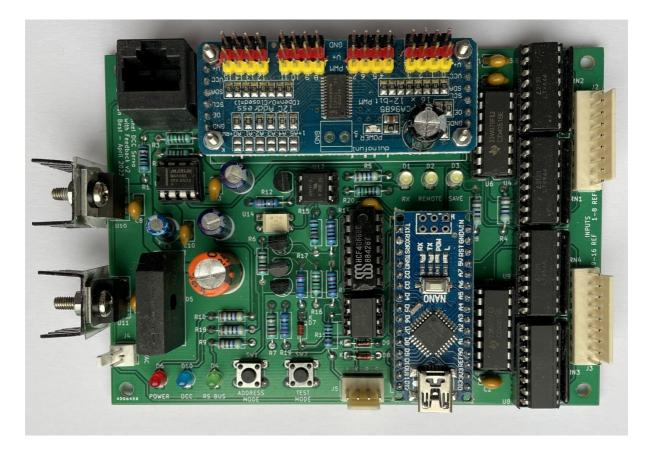
To enable the board to be easily configured I built a setting module. This connects to each servo board via an ethernet cable and allows each servo to be precisely set up before being saved to the module.
