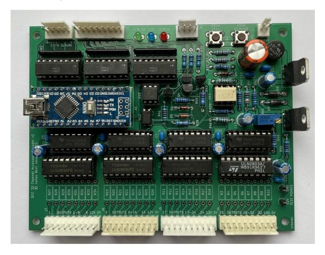
Finally I designed a servo control module which can control 16 channels of servos. Each servo can have its rotation, speed and type of effect set for each direction. There are currently 18 different effects which range from linear motion to various types of bounce. I use this for controlling a range of devices from semaphore signals to gates to a private siding. There are 16 channels of opto-isolated feedback which I use to confirm, via microswitches, that the servo has moved.
