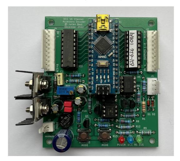
I then added a 32 channel accessory decoder. Each output can individually sink 500mA but I primarily use it for driving LEDs. The current can be set by inserting appropriate resistors (or none) for each channel.
