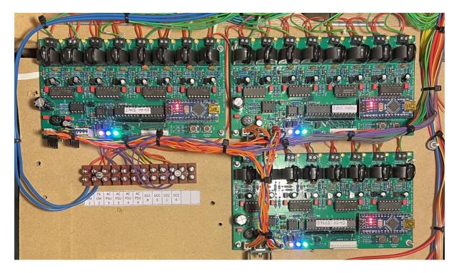
After the success of this module I thought I could expand the concept to include other types of accessory decoders with feedback. This is a 16 channel accessory decoder with feedback. The feedback can confirm that the accessory decoder has responded.
